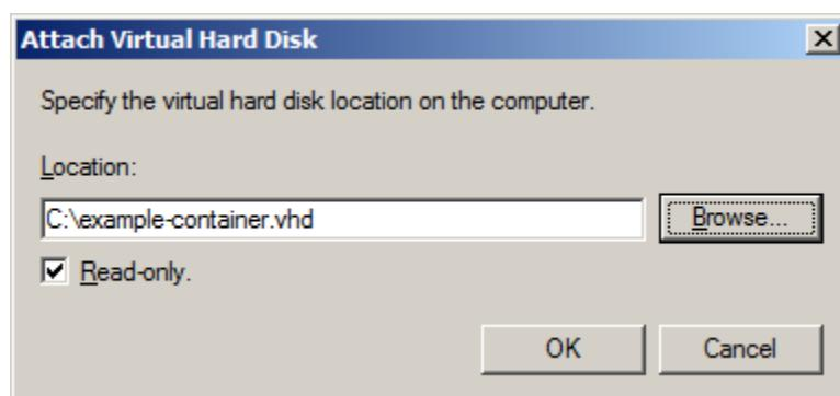
Be sure to check the "Read-only" option when attaching the VHD
